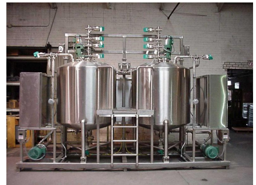
Batch / Weighing System Skid
